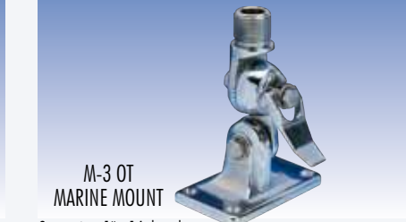
M-3 OT MARINE MOUNT Connection: 1" x 14 threads Dimension L x W x H: 60 x 95 x 130 mm Weight (approx.): 860 gr Material: Chromed brass, Stainless steel hardware M-3 OT marine mount ..... P/N 2503606.00
