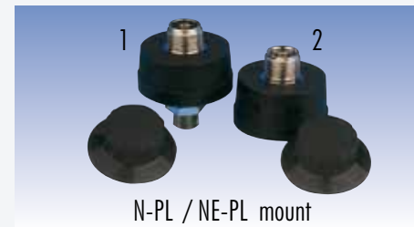
N-PL / NE-PL mount Overall Size: Ø 42 mm Mounting Hole: N-PL Ø 12.5 mm; NE-PL Ø 10 mm Materials: Chromed Brass, Nylon, Rubber Connection: UHF-female 1. N-PL w/Cap ..... P/N 2500502.05 2. NE-PL w/Cap Low profile ..... P/N 2500602.05
