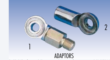
ADAPTORS 1. SB 3/8 adaptor: 3/8 mount to DV joint whip ..... P/N 2506606.00 2. SP 3/8 adaptor: 3/8 whip to DV joint mount ..... P/N 2506706.00 All available in black version
