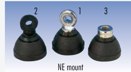
NE mount Overall Size: Ø 36 mm Mounting Hole: Ø 10 mm Materials: Chromed Brass, Nylon, Rubber 1. NE Chrome ..... P/N 2500202.01 2. NE Black ..... P/N 2500202.02 3. NE 3/8 ..... P/N 2500202.03
