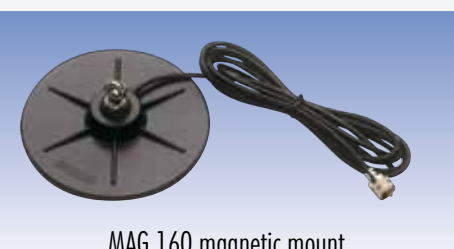
MAG 160 magnetic mount Frequency Range: from DC to 500 MHz Overall Size: Ø 166 mm Materials: Chromed Brass, Nylon, Magnetic rubber Cable: 3.6 m RG 58 / PL 259 R male MAG 160 S ..... P/N 2502802.01 MAG 160 S Black ..... P/N 2502802.02 MAG 160 3/8 ..... P/N 2502802.03 MAG 160 PL ..... P/N 2502802.05
