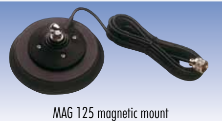
MAG 125 magnetic mount Frequency Range: from DC to 500 MHz Overall Size: Ø 127 mm Materials: Ferrite magnet, Chromed Brass, Nylon, Rubber protection Cable / Connector: 3.6 m RG 58 / PL 259 R male MAG 125 S ..... P/N 2502602.01 MAG 125 S Black ..... P/N 2502602.02 MAG 125 3/8 ..... P/N 2502602.03 MAG 125 PL ..... P/N 2502602.05
