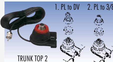
Type: Trunk mount Cable / Connector: 5.5 m RG 58 / UHF-male Connection: UHF-female, 3/8" Thread or DV joint 1. PL or DV chrome ..... P/N 2504406.12 1. PL or DV black ..... P/N 2504407.13 2. PL or 3/8 Chrome ..... P/N 2504406.14 2. PL or 3/8 Black ..... P/N 2504407.14
