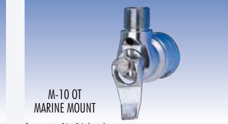
M-10 OT MARINE MOUNT Connection: 1" x 14 threads Fixing diameter: 1" Weight (approx.): 600 gr Material: Chromed brass, Stainless steel hardware M-10 OT marine mount ..... P/N 2503406.00
