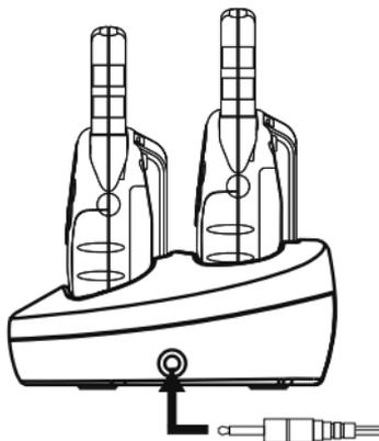
➔ **Important:** The charging is not stopped automatically - be sure to terminate the charging in time in order to avoid overcharging of the battery packs!
