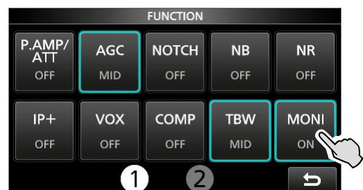
5. Rotate **(MULTI)** to adjust MONITOR to the clearest audio output between 0% and 100%, while speaking at your normal voice level.
