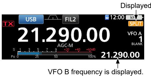
3. While holding down **XFC**, set the operating frequency offset between transmit and receive.
