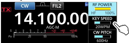
4. Rotate **(MULTI)** to set the key speed to between 6 and 48 Words Per Minute (WPM).
