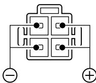
Connects to a regulated DC power source of 13.8 V DC  $\pm 15\%$  through the supplied DC power cable.
