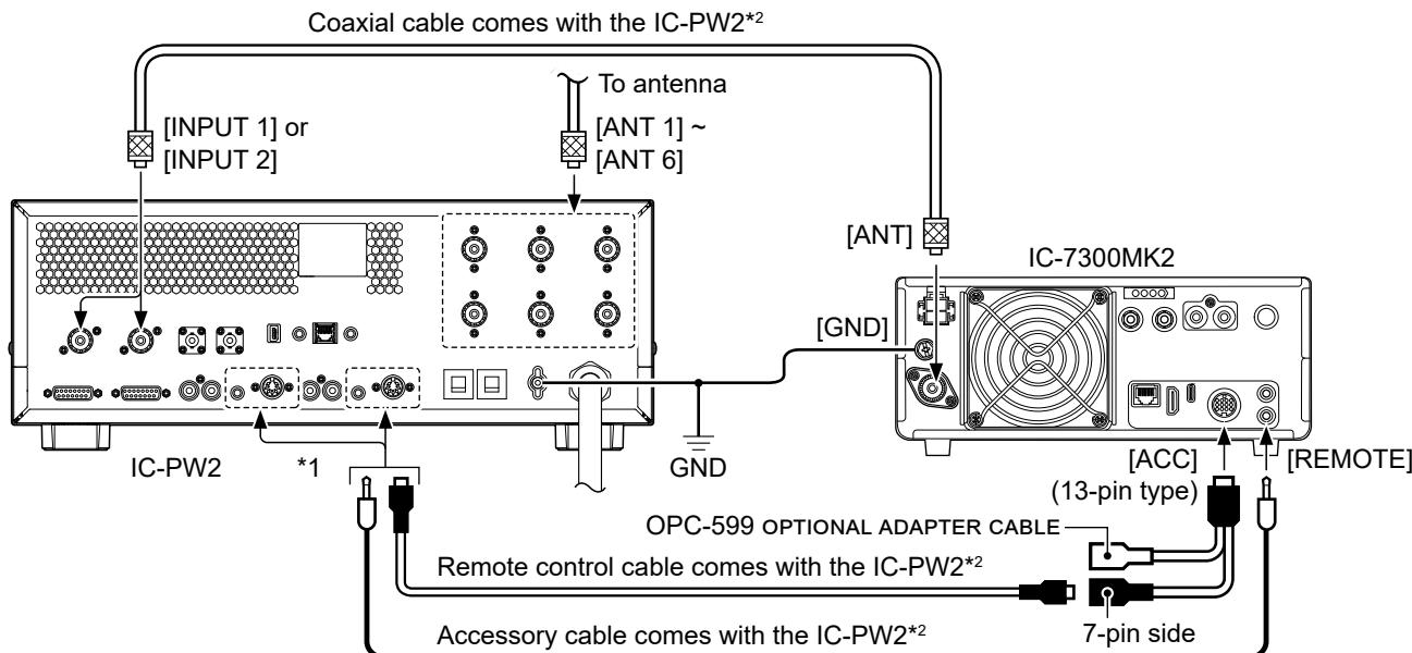
\*1 When you connect a coaxial cable to [INPUT 1], connect to [REMOTE 1] and [ACC 1].
