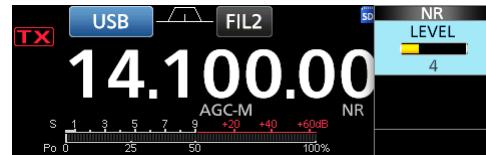
① Adjust to a higher level to increase the reduction level, and a lower level to decrease it.
