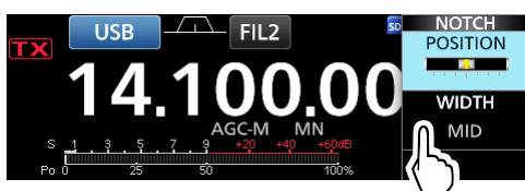
3. Rotate  $\circledcirc$ MULTI slowly to manually attenuate the frequency.
