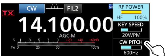
4. Rotate **(MULTI)** to set the CW pitch to between 300 and 900 Hz (in 5 Hz steps).
