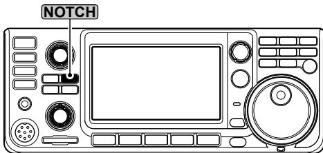
① Pushing [NOTCH] changes between "AN (Auto Notch)," "MN (Manual Notch)," and OFF.
